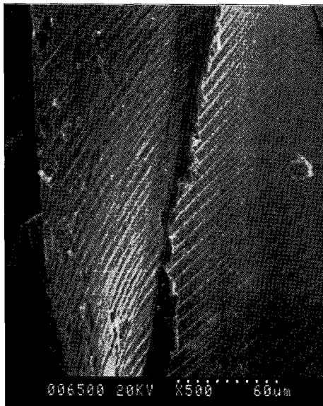
Figure 2. Photomicrograph of a HEROShaper instrument in group 2 (before fatigue testing) showing the presence of manufacturing defects such as metal roll-over and machining marks (original magnification, \times 500 ).
