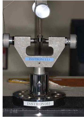
Fig. 2. Pull out test in universal test machine.
