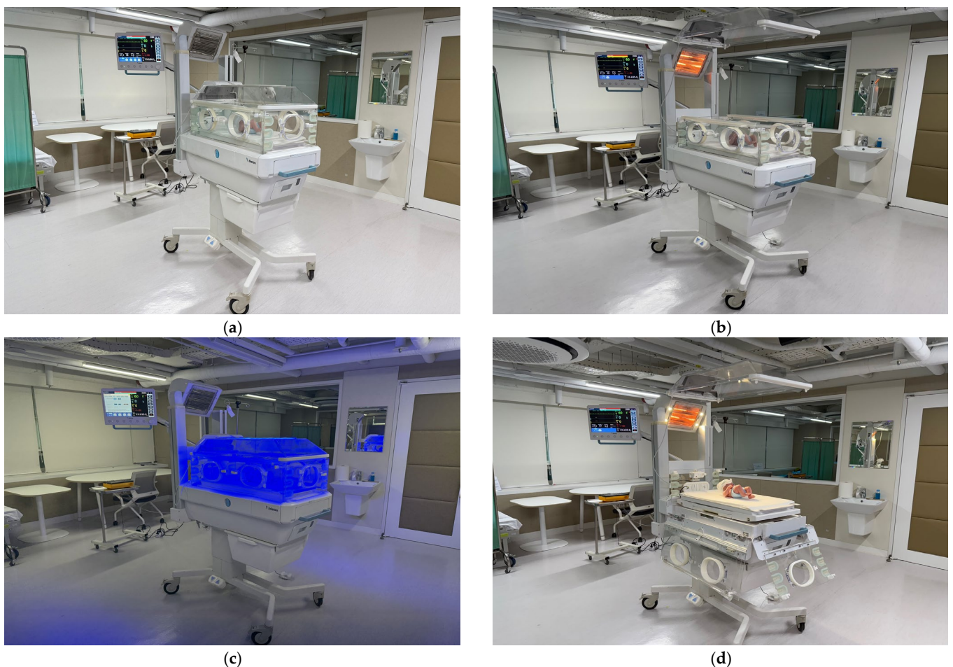
Figure 4. Evaluation environment of the multi-functional neonatal incubator under different operational modes: (a) incubator mode; (b) radiant warmer mode; (c) phototherapy mode; and (d) surgical mode.
