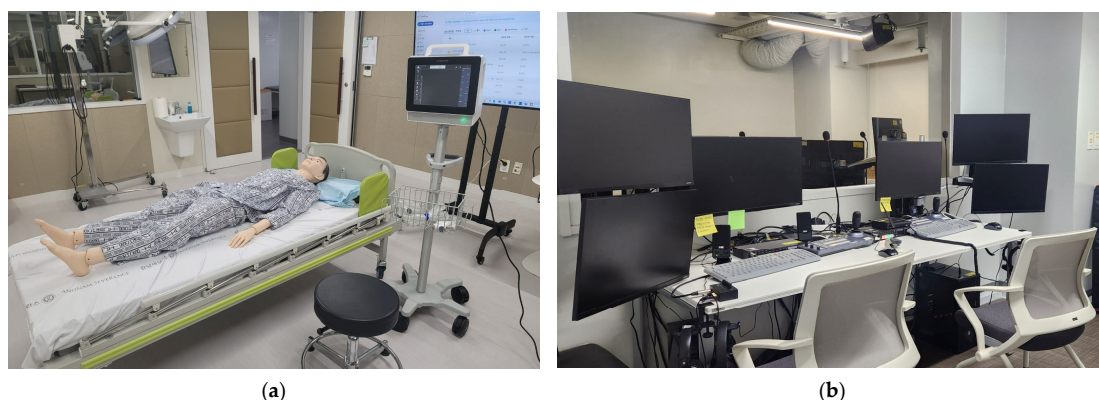
Figure 2. Configuration of the usability test environment: (a) Test room designed to simulate an actual operating room setting; (b) Observation room equipped for real-time monitoring and data recording.
