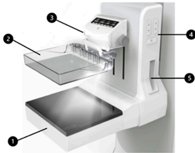
Figure 2. Main imaging components of the MammouS-N system. 1. Breast Ultrasound Scanner: Automatically captures images across the compressed breast surface. 2. Breast Compression Device: A compression plate that ensures firm contact between the breast and the ultrasound probe. 3. Manual Compression Adjustment Handle: Allows manual raising and lowering of the compression device. 4. Breast Stabilization Device Control Console: Control panel for operating the breast stabilization system. 5. Patient Stabilization Handle: A support handle for the patient to hold during the imaging process.
