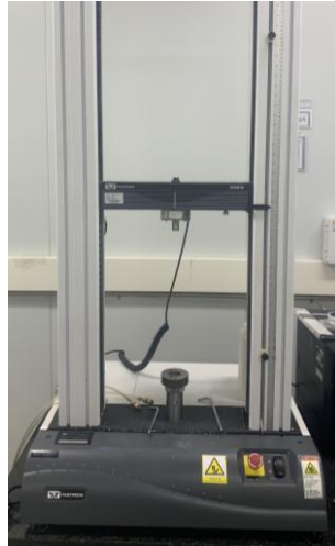
Figure 4. Dual column universal testing machine for static compression test (INSTRON 3365, Instron Corporation, MA, USA).
