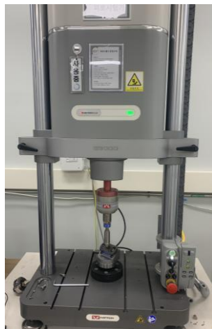
Figure 5. Linear-torsion testing machine for dynamic loading test (INSTRON E3000, MA, USA).
