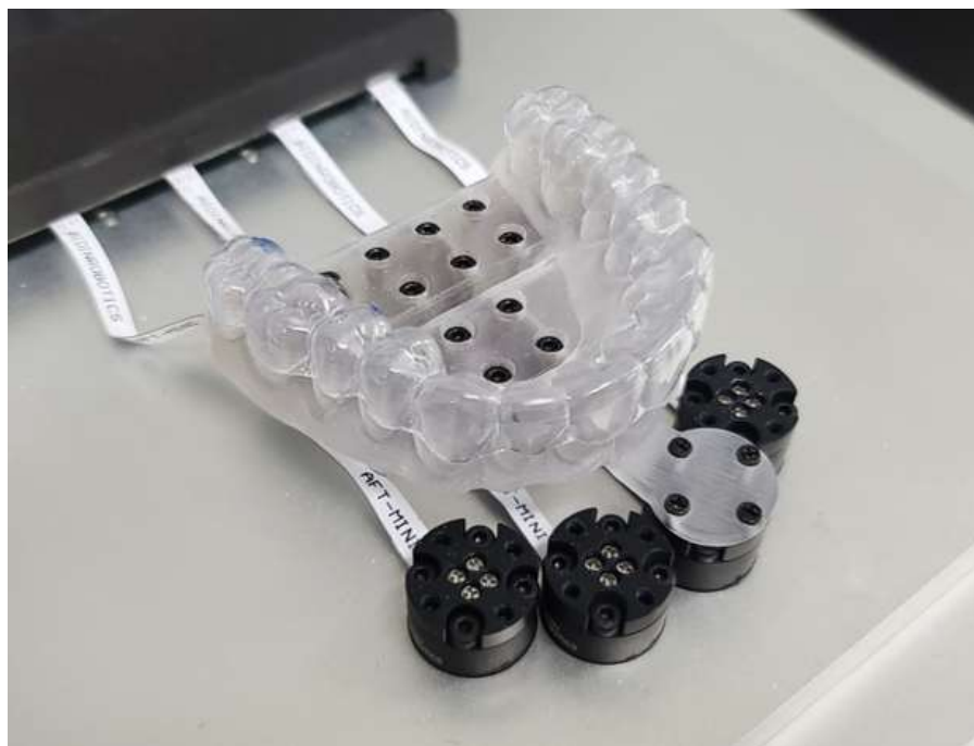
Fig 2. Force/Torque measuring equipment with Miniature 6 Axis F/T Sensor
