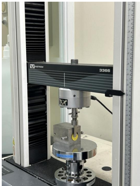
Figure 3. Universal testing machine (Model 3366; Instron Co., Norwood, MA, USA)
