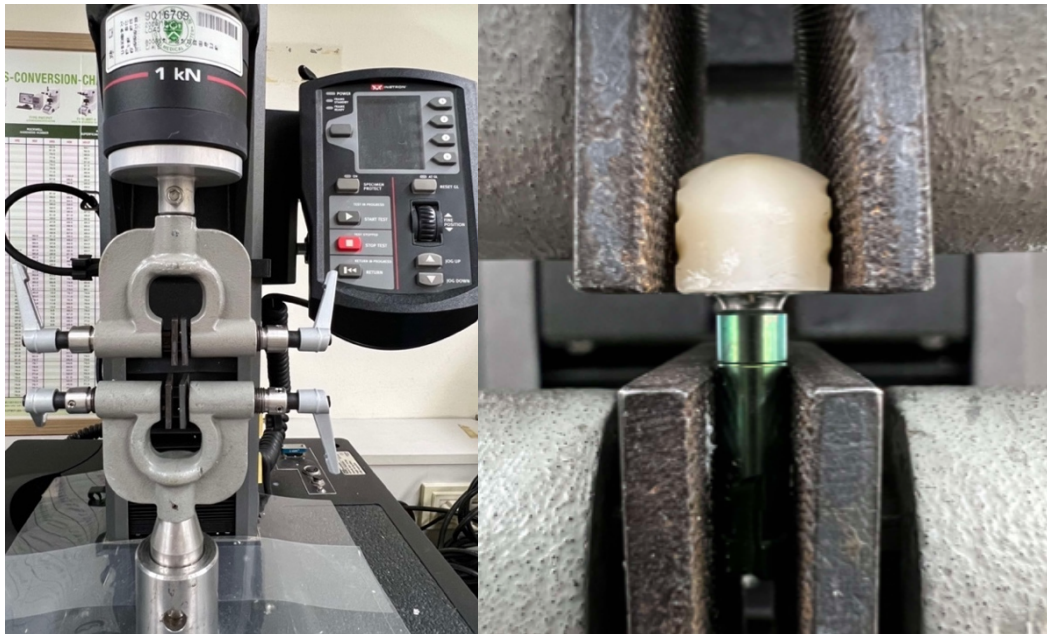
Figure 4. Universal Testing Machine (5942 model, Norwood, MA, USA) used for measuring pull-out force at a crosshead speed of 1 mm/min in this experiment
