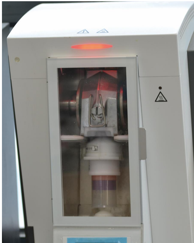
Figure 2. The injection machine (IvoBase Injector; Ivoclar Vivadent AG, Schaan, Liechtenstein) used for the fabrication of Group HEA specimens.
