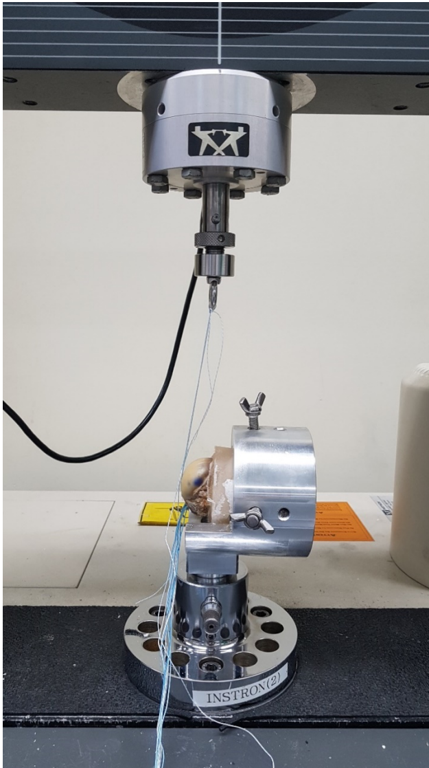
Figure 3 Pulling the sutures with the Instron (Instron 3366, Instron Co., Ltd, Norwood, MA)
