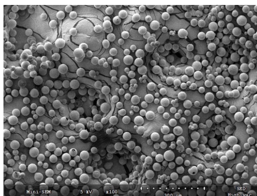
Figure 2. SEM image of CaHA in DClassy (CGBIO Inc., Seoul, Republic of Korea).
