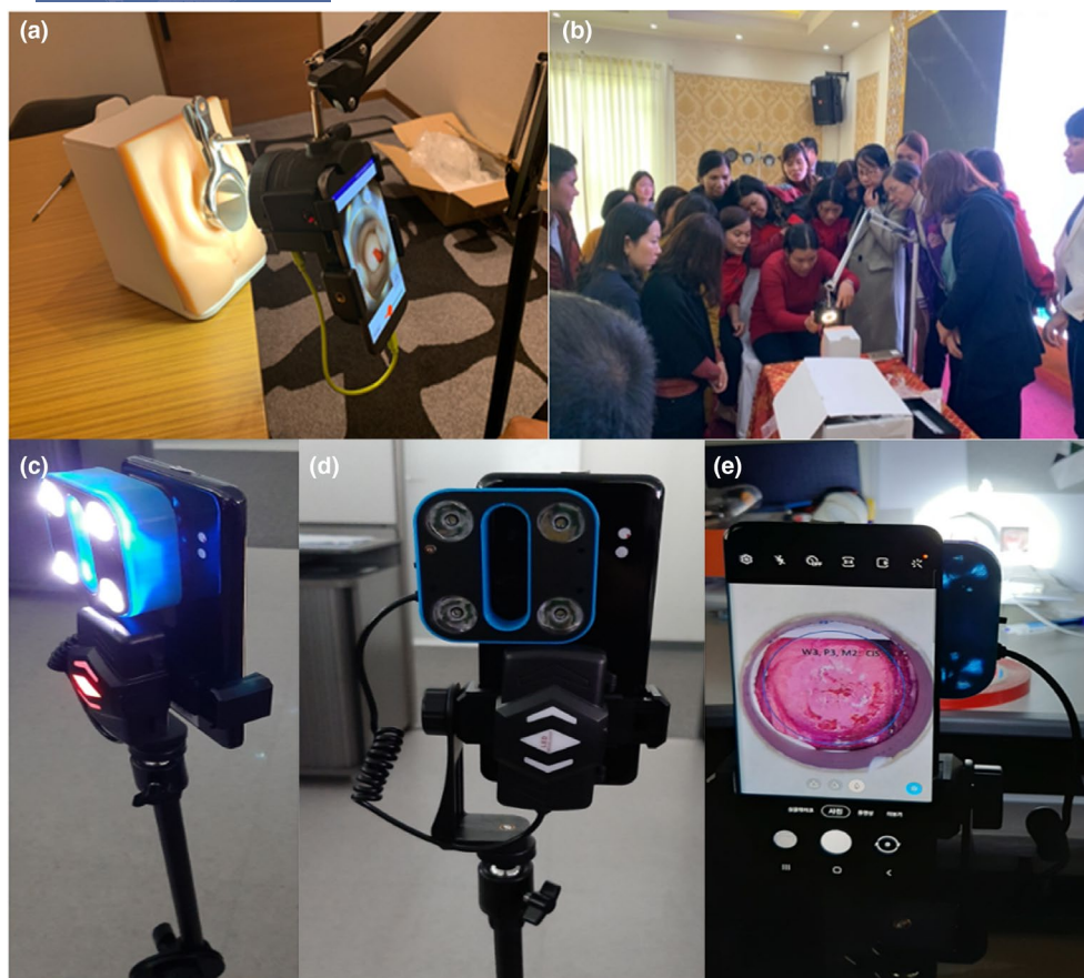
FIGURE 1 Upcycled smartphone-based colposcopy. (a) First prototype of swing type smartphone-based colposcopy. (b) Training of community health workers for obtaining colposcopy images. (c–e) Upgraded version of tripod type smartphone-based colposcopy with light-emitting diode (LED) flashlight.
