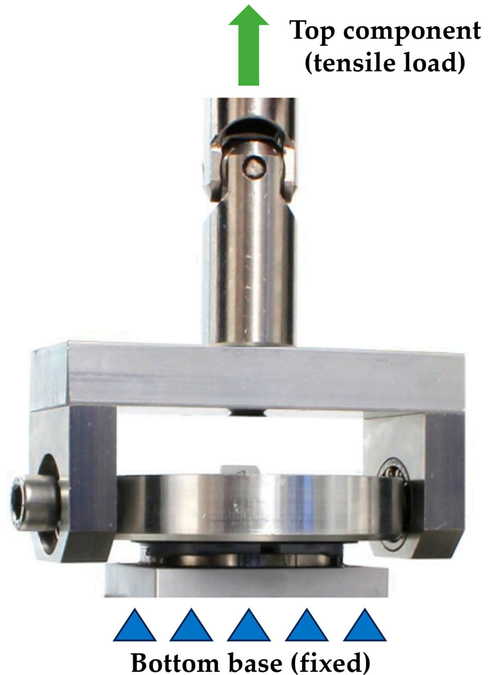
Figure 2. The setup for the static disassembly test in the tensile loading direction.
