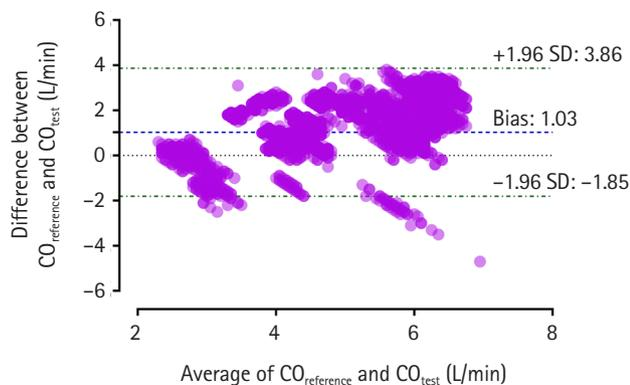
**Figure 4.** Bland-Altman plot of cardiac output (CO) measured by two devices (test: HemoVista, reference: FloTrac). Bias was defined as the average of the differences in CO measured between the reference device and the test device. The percentage error was 55.8%. SD: standard deviation.
