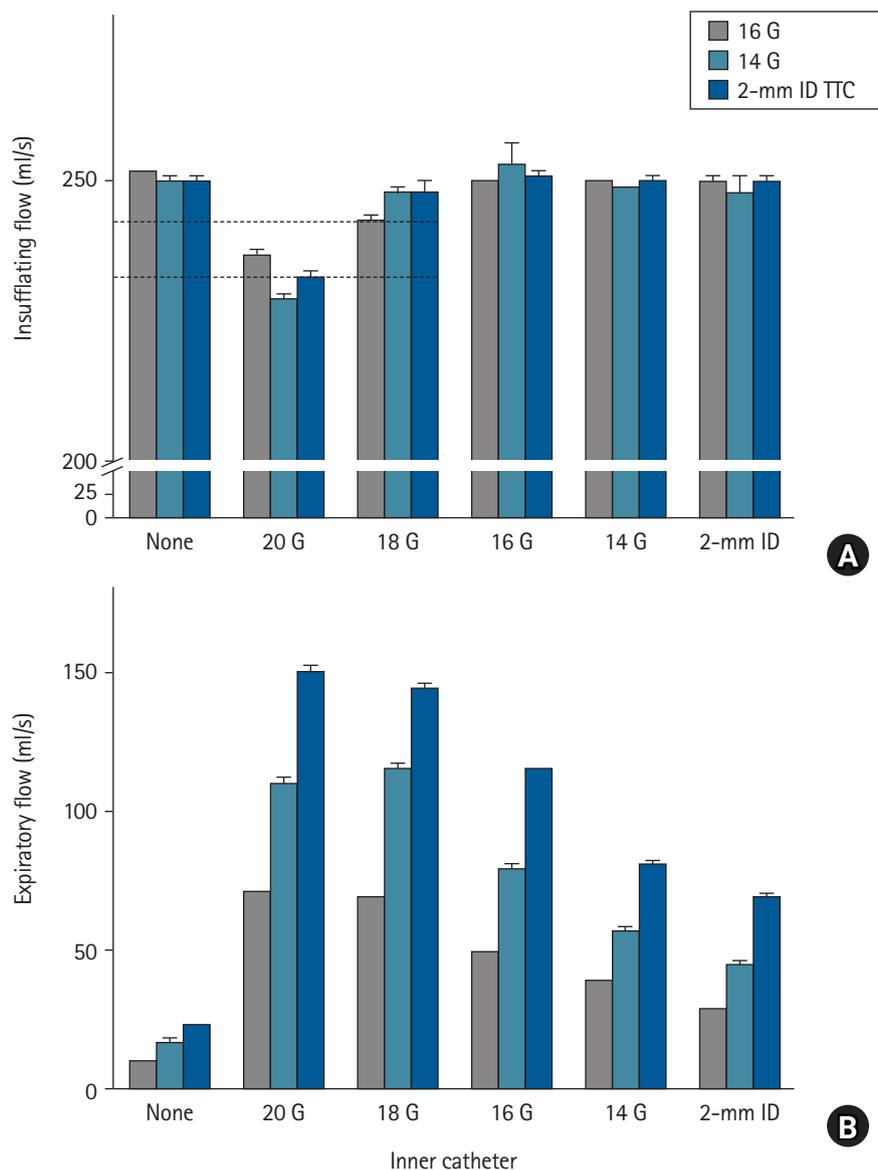
**Fig. 4.** (A) Insufflating and (B) expiratory flows measured using insufflation catheters of 16 G, 14 G, and 2-mm ID in conjunction with 20 G, 18 G, 16 G, 14 G, or 2-mm ID TTC inserted into the connecting port of the T-connector (inner catheter) of the modified Rapid-O2 at an oxygen flow rate of 15 L/min. None indicates the absence of inner catheters. ID: inner diameter. TTC: transtracheal catheter. N = 4 in each group.
