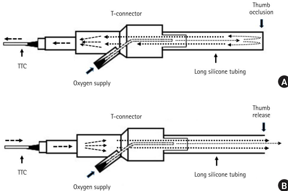
**Fig. 2.** (A) Schematic illustration of insufflating and (B) expiratory gas flows in the modified Rapid-O2. Expiration is induced by releasing the thumb at the end of the silicone tubing and is enhanced by negative atmospheric pressure via the Venturi effect. TTC: transtracheal catheter.
