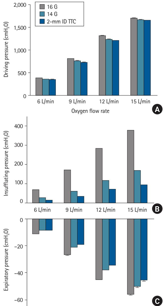
**Fig. 5.** (A) Driving, (B) insufflating, and (C) expiratory pressures through the 16 G, 14 G, and 2-mm ID insufflation catheters measured with an 18 G inner catheter at oxygen flow rates of 6, 9, 12, and 15 L/min. ID: inner diameter.  $N = 4$  in each group.
