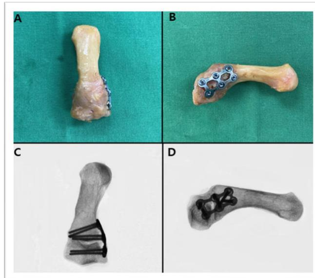
Figure 2. Radially fixed group. Specimen preparation after radial plating (a, b) and radiographic scanning (c, d).
