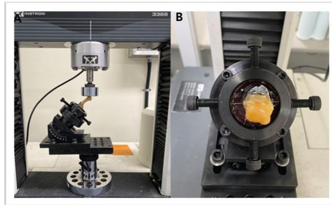
Figure 3. Cantilever bending test setup. (a) Long axis of the metacarpal bone set at 45° to the vertical loading axis and (b) Rounded specimens were clamped by screws.
