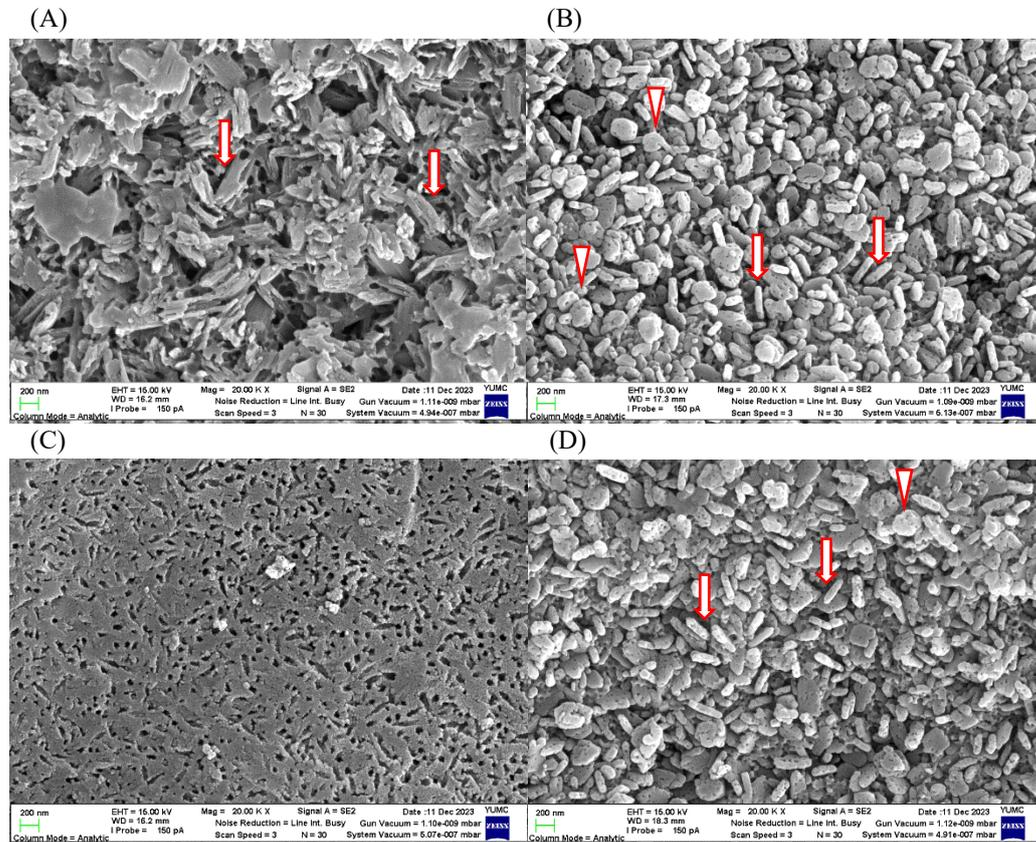
**Figure 3. SEM image of glass ceramic etched with 4% HF for 30s. (A) IPS e.max<sup>®</sup> CAD after firing (B) CEREC Tessera<sup>™</sup> after firing (C) IPS e.max<sup>®</sup> CAD before firing (D) CEREC Tessera<sup>™</sup> before firing (magnification x20,000)**
