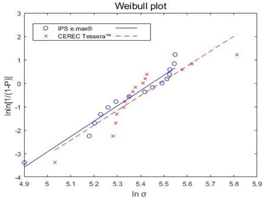
**Figure 2. Weibull plot for glass ceramic.**
