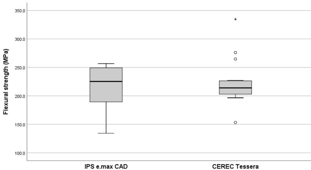
**Figure 1. Box plot of flexural strength of glass ceramic.**
