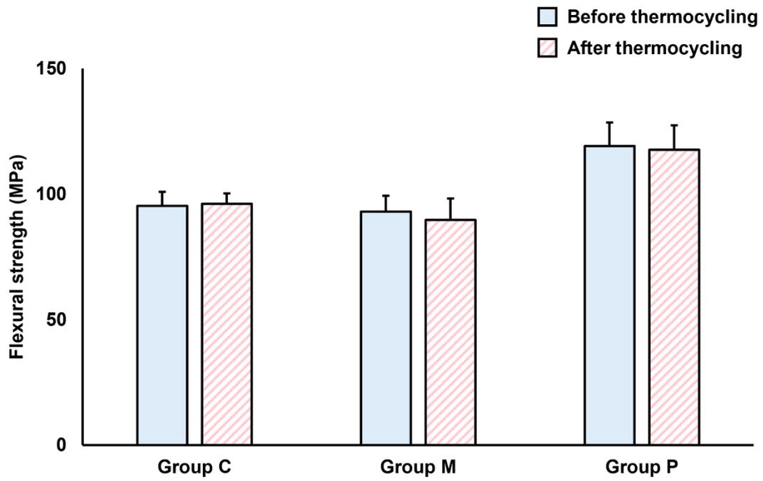
**Figure 2.** Comparison of the flexural strength for the three specimen groups before and after thermocycling. Groups C, M, and P represent the conventional, milling, and 3D printing fabrication methods.
