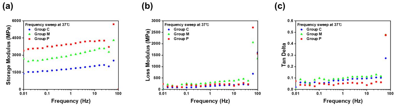
**Figure 4 :** Dynamic rheological properties as a function of the frequency for Groups C, M, and P at 37 °C.
