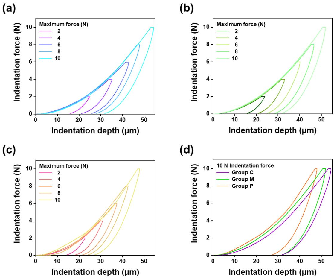
**Figure 5** : Pressure-indentation characteristics in the nanoindentation tests. Indentation deformation behavior of the resins as a function of various indentation loads of 2–10 N (a) Groups C, (b) M, and (c) P. (d) Comparison of the force-depth curves of Groups C, M, and P at an indentation load of 10 N.
