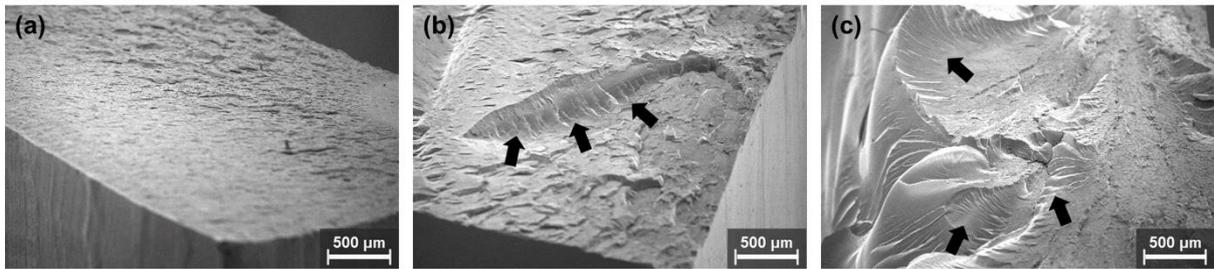
**Figure 6** : SEM images ( $\times 40$  magnification) of the fracture surfaces of each material. (a) Group C. The smooth and even surface. (b) Group M. Arrows indicate the jagged, rough appearance, and partially torn aspect. (c) Group P. Arrows indicate stretching and tearing features.
