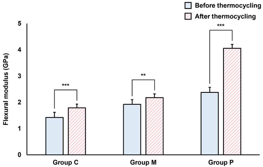
**Figure 3.** Comparison of the flexural modulus for the three specimen groups before and after thermocycling. Groups C, M, and P represent the conventional, milling, and 3D printing fabrication methods. Comparison among groups is expressed as \* $P < .05$ , \*\* $P < .01$ , \*\*\* $P < .001$ , asterisks and horizontal bars indicate statistically significant differences before and after thermocycling.
