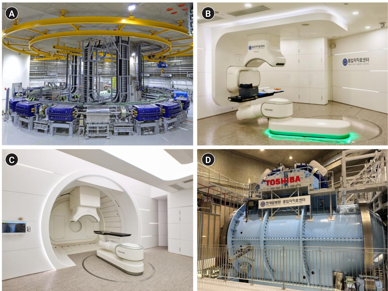
**Fig. 3.** (A) Synchrotron for carbon ion acceleration, (B) fixed treatment room, (C) gantry treatment room, and (D) inner parts of gantry with a superconducting magnet.
