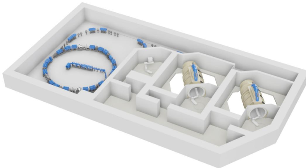
Fig. 1. Three-dimensional layout of the accelerator and three treatment rooms (i.e., fixed- and two gantry-type rooms) at the Yonsei Cancer Center (from left to right).
