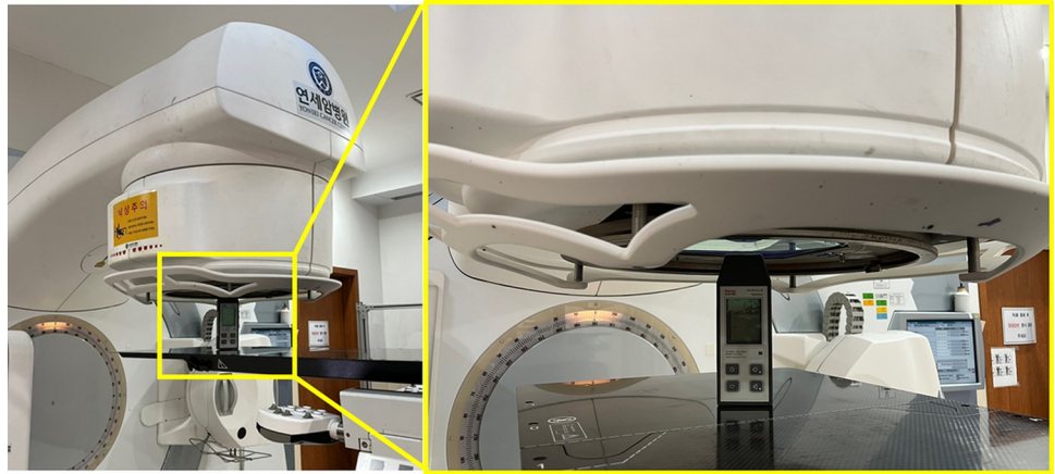
Fig 2. Set-up of HPGe detector for spectroscopic measurements.
