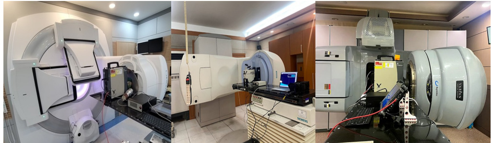
Fig 1. Set-up of HPGe detector for spectroscopic measurements.
