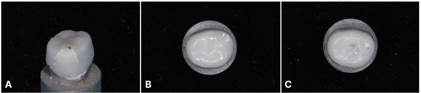
Fig. 3. Fracture patterns observed after chewing simulations. (A) Among the 12 specimens made of GP, one exhibits a large vertical fracture, (B, C) Whereas in the case of MD, two out of the 12 specimens show chipping-type fractures.
