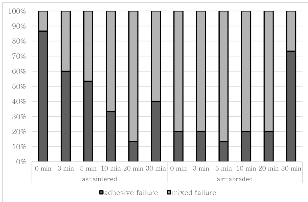
Figure 7. Failure mode percentage for as-sintered and air-abraded zirconia surfaces.
