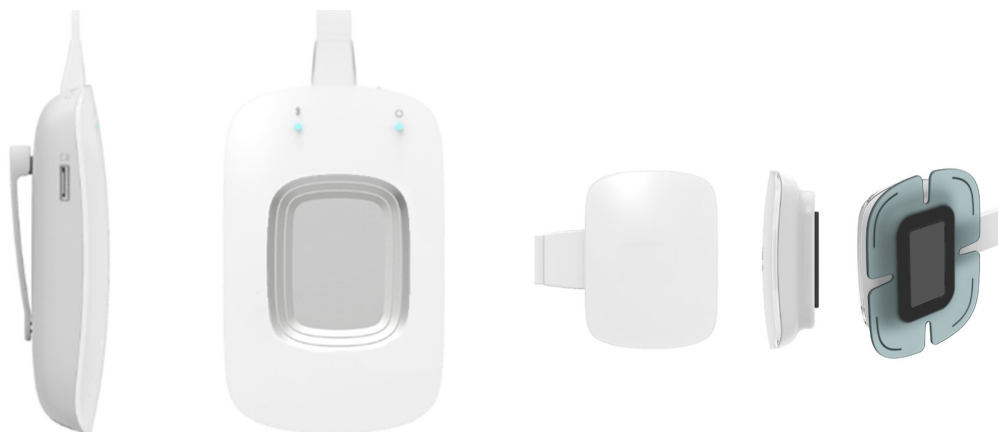
Figure 3.8 Design sketch of the wearable bladder monitoring system
