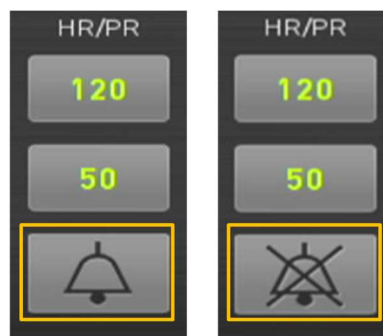
Figure 17. Audible Alarm Stop Button for Each Parameter. (left: audio alarm activated state, right: audio alarm stopped state)
