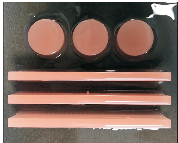
Fig. 2. Three-dimensional printed flexible denture resin specimens.
