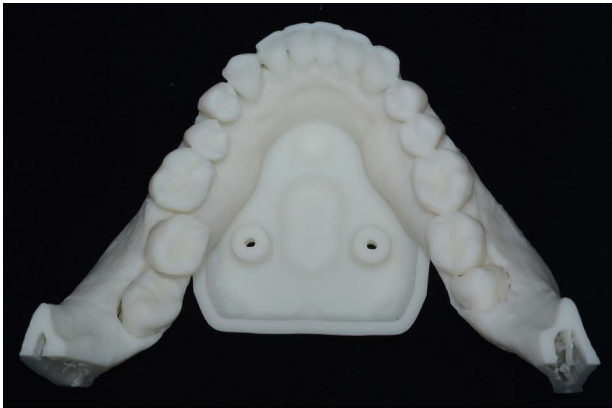
Figure 1. The 3D printing model for surgical extraction simulation of the impacted lower third molar. The model consists of a mandibular part, dentitions, and a plate for attaching to the mannequins.
