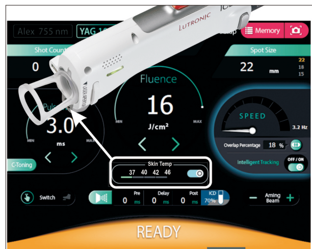
Fig. 2. The GUI (touch screen) of the long-pulsed Nd:YAG laser used in the present study with the skin temperature indicator (white bounding box) and the infrared temperature sensor indicated on the superimposed handpiece (white arrow) (Courtesy, Lutronic Corporation, Goyang, South Korea).
