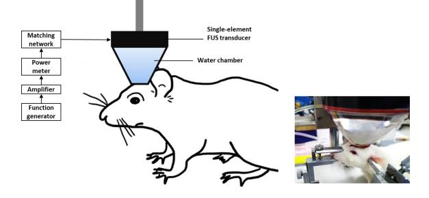
Figure 1. Schematic diagram of focused ultrasound experimental set-up.
