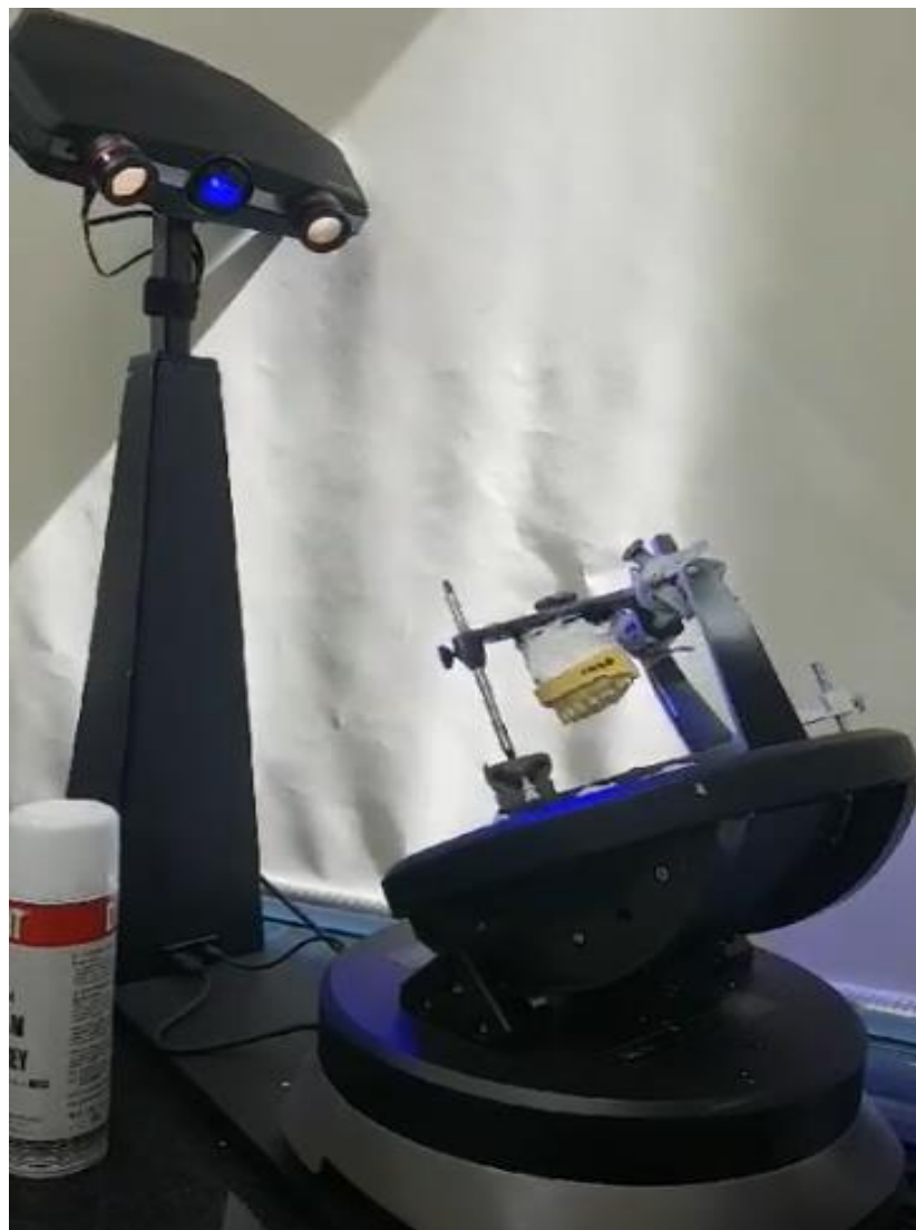
Figure 5. Scanning of conventional mounting models using the industrial scanner. Powder spray was applied to the surface of articulator to prevent diffused reflection that may occur during scanning.
