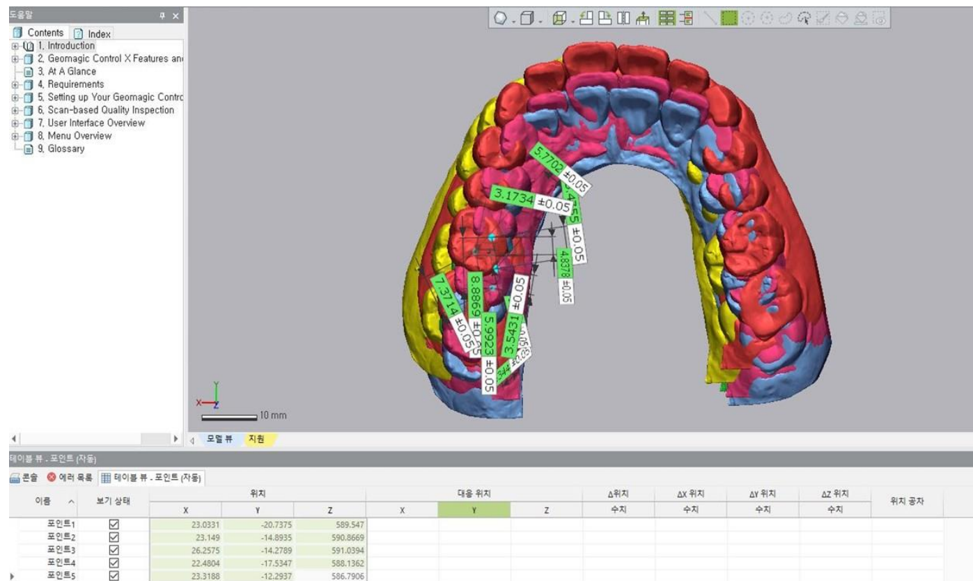
Figure 11. Finding coordinates of the target points and distance between the target points via Geomagic control X software.
