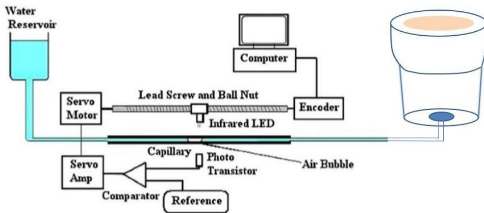
Fig 1. A Schematic diagram of the fluid flow measurement system (Nanoflow; IB systems, Seoul, Korea) modified from the original publication (Kim, et al., 2010; Kim, et al., 2013).
