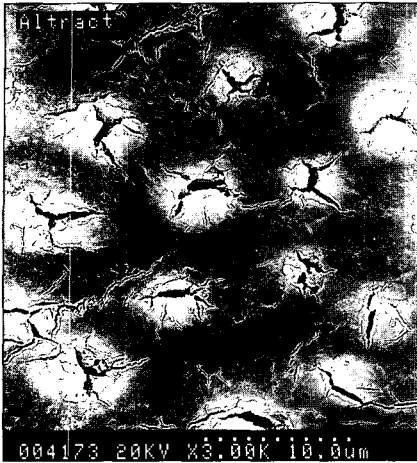
Fig. 6. SEM of dental surface exposed to Altract for 2 minutes.
