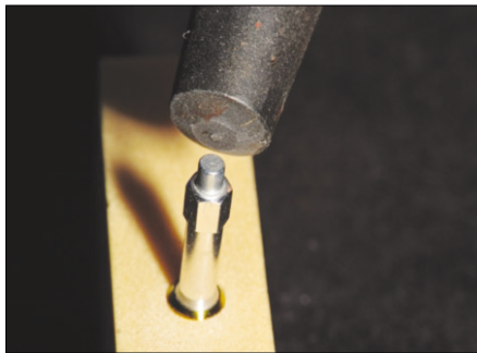
Fig. 3. Measurement of ISQ value using resonance frequency analysis.
