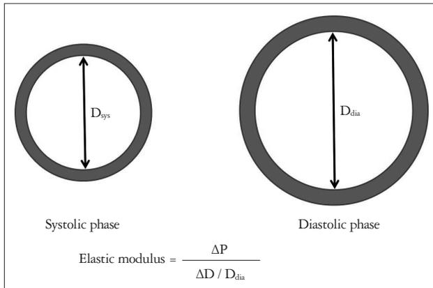
**Fig. 1.** Definition of terms used for the calculation of elastic modulus index.
