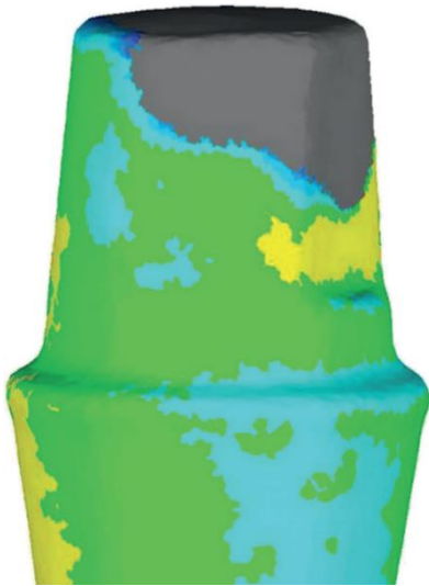
Fig.11 Superimposed image between intact and damaged abutments. Gray area shows volume loss incurred from drilling
