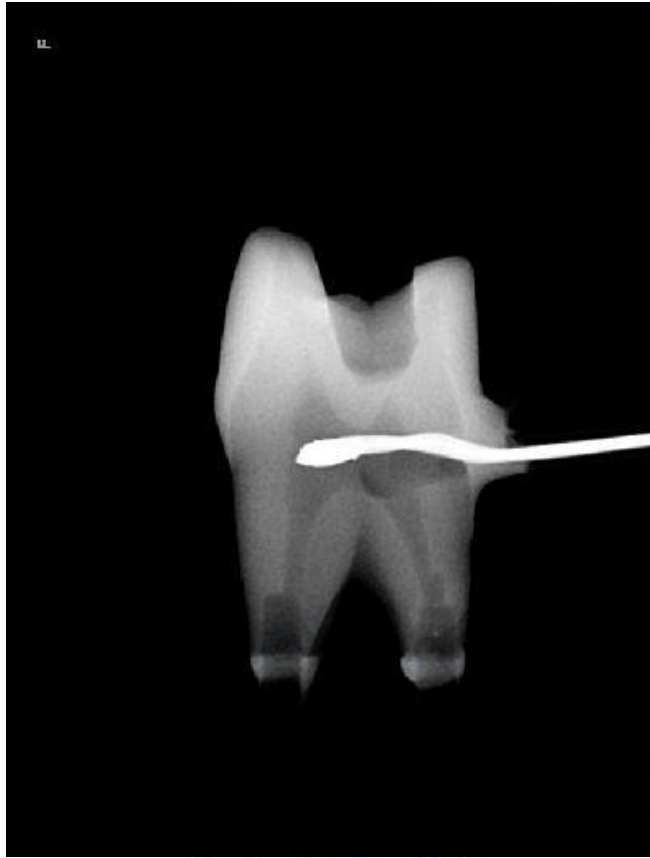
Fig. 2. X-ray of the premolar with a thermocouple and plastic tubes.
