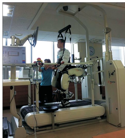
Fig. 1. Lokomat, a robot-assisted gait training system, consisted of robotic gait orthosis, body weight support, and treadmill.
