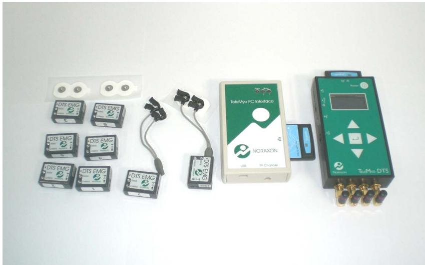
Figure 3. Wireless surface electromyography (TeleMyo DTS).
