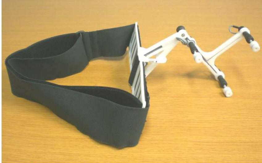
Figure 2. Triple markers for the measurement of spine motions.
