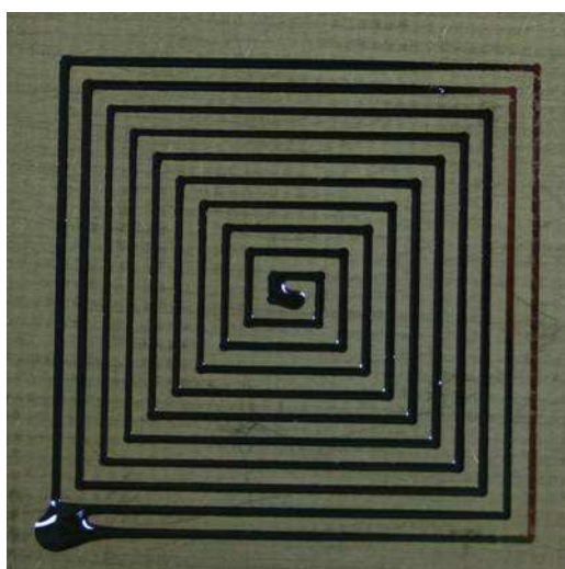
Figure 5-7 Pattern result by using Type I lens (FR4; Double-faced coating of Cu)
