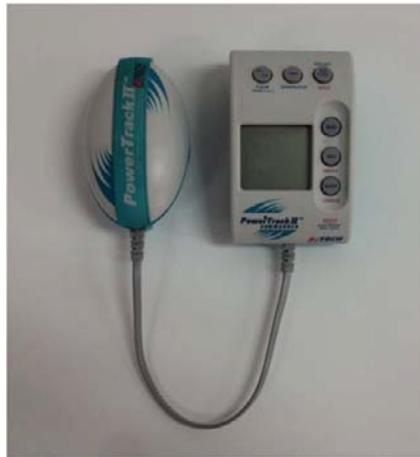
Figure 3. PowerTrack II™ Commander dynamometer.
