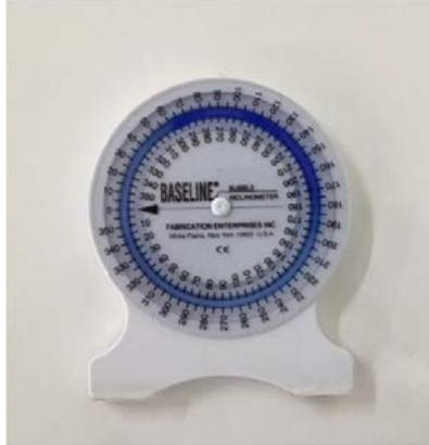
Figure 2. Inclinometer.
