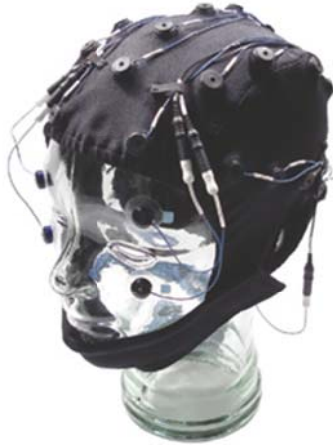
Figure 2.3. A typical electrode cap used in EEG recording systems (source: www.neuroscan.com).
