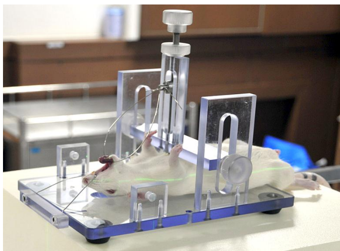
Fig. 4. Customized fixation device for local irradiation.
