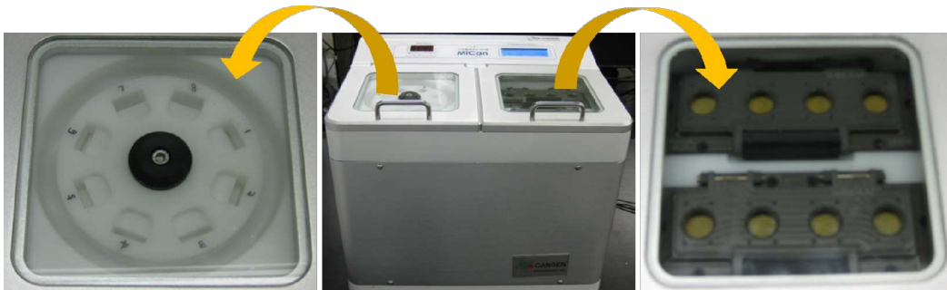
Figure 2.5. Measurement humidity controlled chamber
