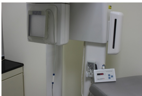
Figure 1. DAP ionization chamber was placed in front of X-ray source of CBCT unit.
