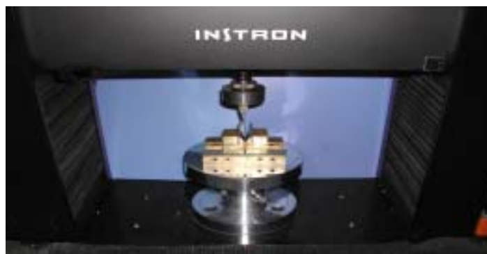
Fig. 5. Photograph of test instrument for 3 point bending test
