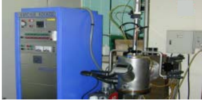
Fig. 1. Arc melter used in this study for manufacturing Ti-Ag alloys
