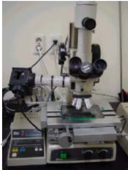
Fig. 3. Apparatus for measuring linear change of impresssion materials (Mearsurescope MM-II, Nikon, Tokyo, Japan).
