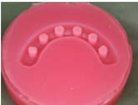
Fig. 2. Silicone mold for wax pattern.
