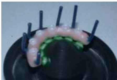
Fig.6. The wax pattern before investing.
