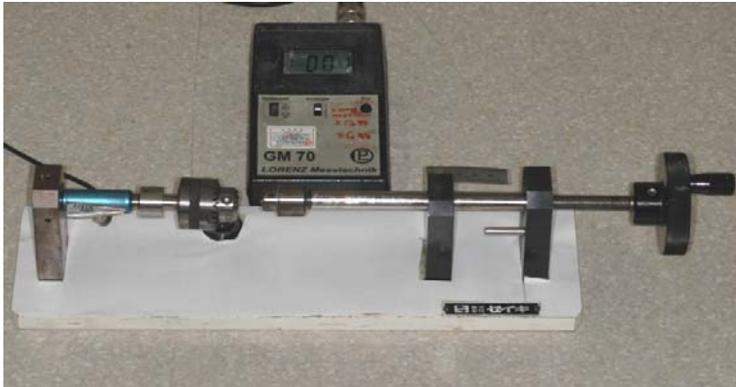
Fig.3. Digital strain gauge(Amplifier GM 70, Messtechnik co., Alfdorf, Germany)
