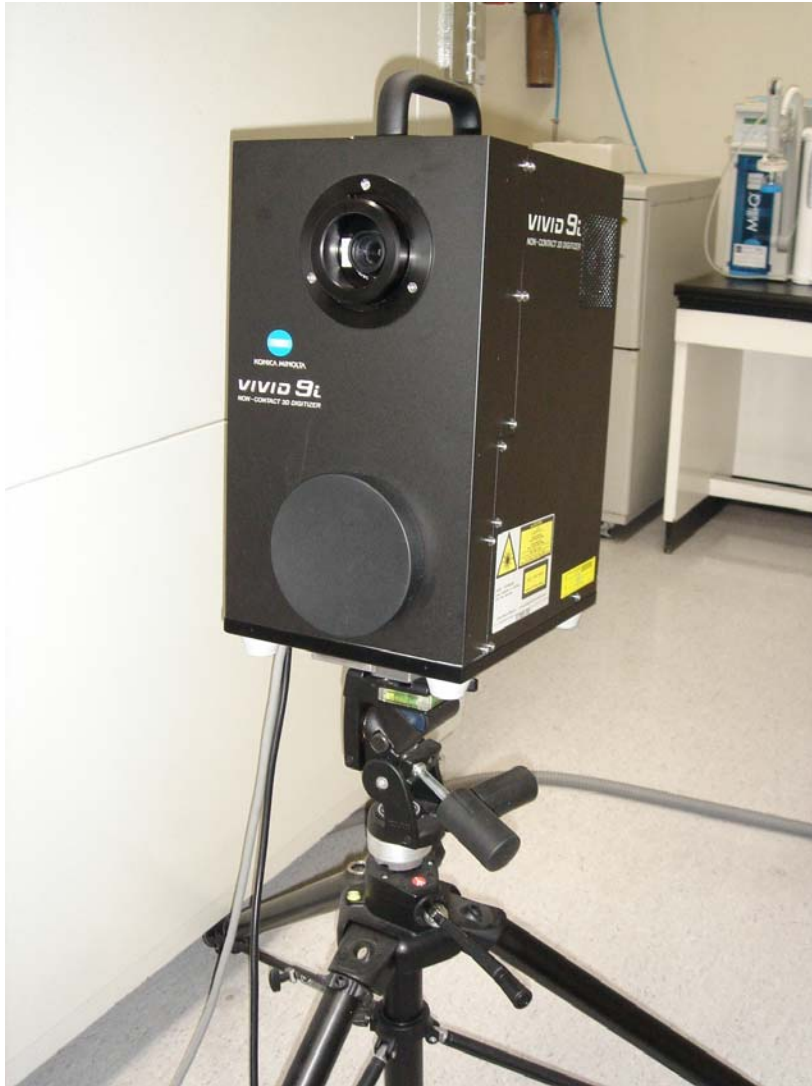
Figure 1. Vivid 9i laser scanner (Minolta, Tokyo, Japan), which emits a harmless Class I laser beam (rated safe for eyes by the US Food and Drug Administration; maximum 30 mW at 690 nm).
