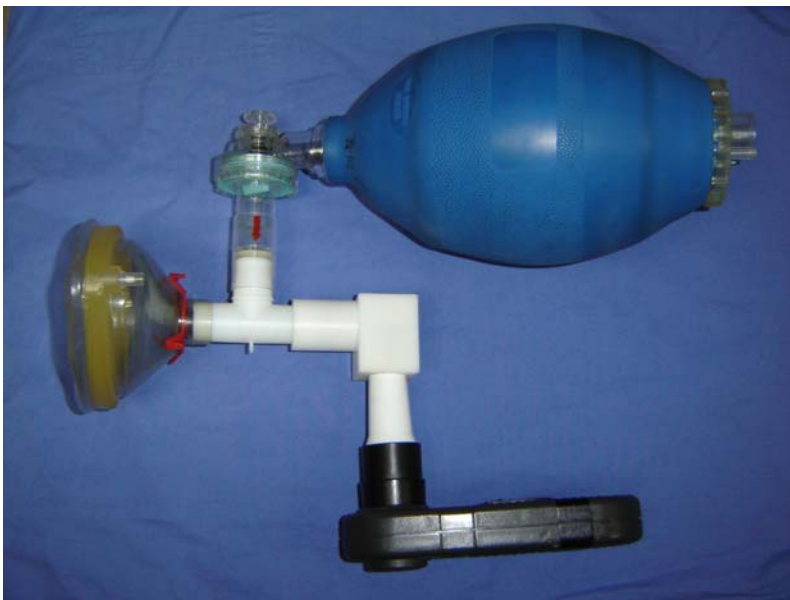
Fig. 3 A fully assembled apparatus for measuring MIC-device: A resuscitation bag is connected to the external control device
